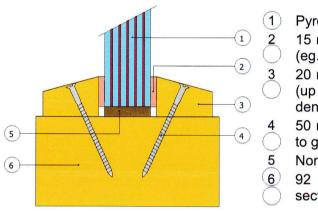
Pyroguard El60 INT or Pyroguard El60 EXT glass 15 mm by 3 mm ceramic fibre based glazing tape (eg. 'K' tape), or Lorient System 36/23
